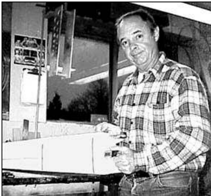
Figure 6 The author testing the newly covered bellows. Each will move easily because of the new, light-weight leather.
