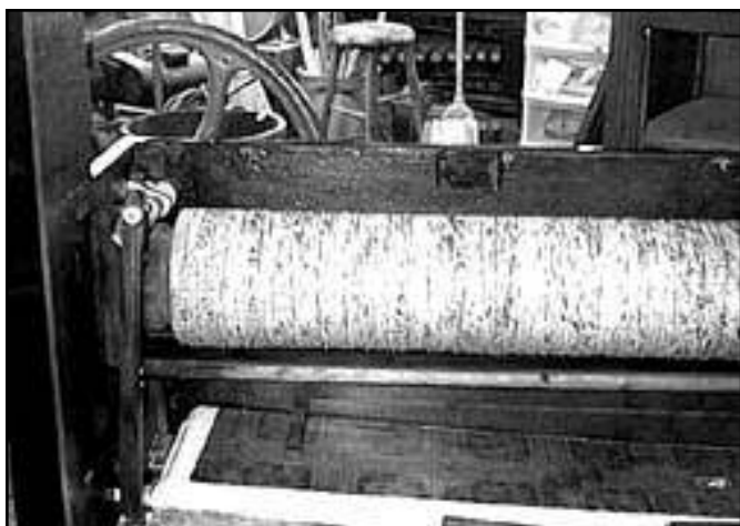
Figure 9 The pinned barrel, restored pump and crank and crank arms now have been put back into the case and ready for testing.
