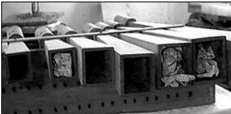
Figure 11 This view reveals the paper "stoppers" in some of the organ's trumpet pipes.
