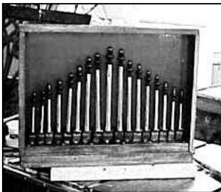
Figure 4 The brass piccolo pipes have been restored and now back in position.
